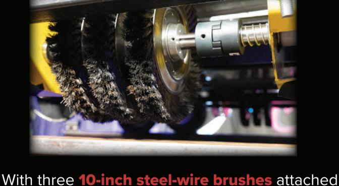
in series on each side of the vehicle, the OnTrack scrub system guarantees a clean polish. The brushes have a 3 month life expectancy and are easily replaceable by releasing the spring-loaded axle.
